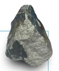
Ferrovanadium alloy is of use as a universal strengthener, hardener, and anti-corrosive agent for different types of steel like tool steel, low-alloy steel, high-strength steel, and other ferrous-based steel.
